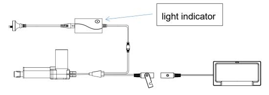
Step1, connect all products according to connection diagram Step2, according to below diagram, press and insert wireless charging panel to pre-cut slot.
