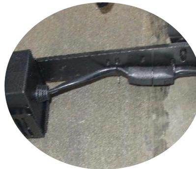
Check motor to-pin cable to transformer for damage and make sure it has a good connection.
