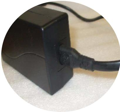
Check power cord for damage and connection to transformer. If the power cord has no damage and its connection to the transformer is good but the green light is not on, then replace transformer.
