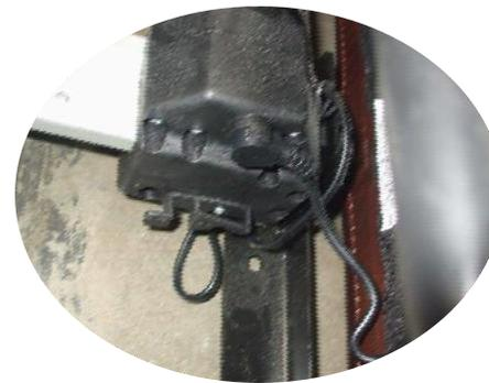
Check power switch cable connection to motor. If you're still without power, it's either the switch or motor. 9 out of 10 times it's the switch.
