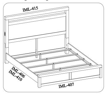
All Beds need to be set up in the exact final location so that after full assembly it will not need to be moved. Moving the bed will cause the support legs to move out of perpendicular (90 degree), weaken the support system, and may allow the bed to collapse.
