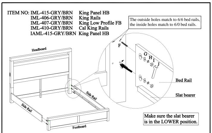
STEP 5: Screw the bolts(F) into HB & FB. Align the bolts with the holes in the end of side rails and attach the side rails to HB & FB using half moon washers(G),lock washers(H) and nuts (I). Then use a hex wrench to tighten all the nuts.
