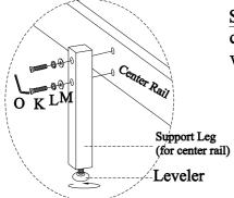
STEP 8: Attach 2 support legs (for center rail) to the center rail using 4 bolts (K), lock washers (L) and flat washers (M). Use an Allen Wrench to tighten all the bolts.
