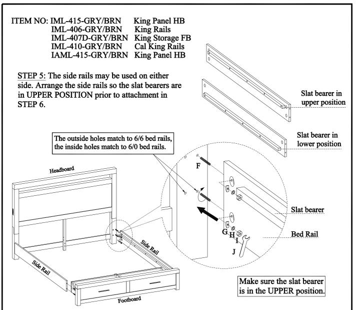
STEP 6: Screw the bolts(F) into HB & FB. Align the bolts with the holes in the end of side rails and attach the side rails to HB & FB using half moon washers(G),lock washers(H) and nuts (I). Then use a hex wrench to tighten all the nuts.
