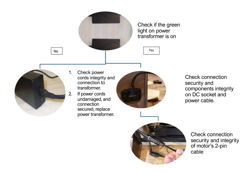
For dual-power recliners, please check connection and integrity of Y-Cable splitter.
