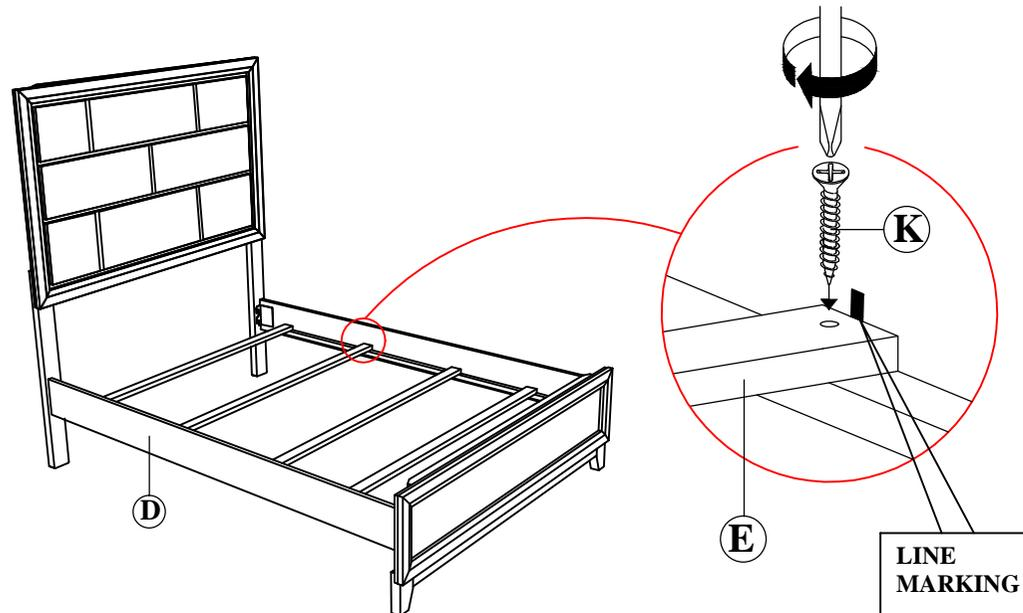
NOTE : MUST TIGHTEN SCREWS PERIODCALLY WITH USE SCREW WILL BECOME LOOSE CHECK TIGHTNESS OF ALL SCREW EVERY 6-8 WEEKS.
