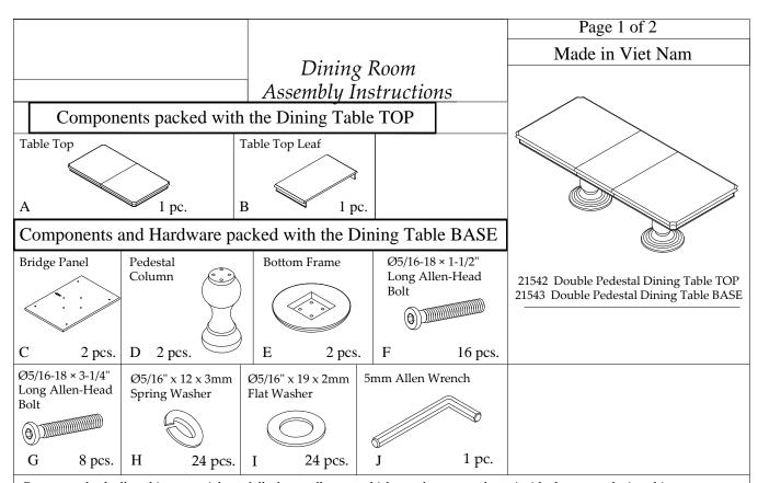
Be sure to check all packing material carefully for small parts, which may have come loose inside the carton during shipment. Separate, count and check all parts against the Components and Hardware List above. Failure to use the correct length bolts in the proper locations may result in an unsafe product and could also cause damage to the parts being assembled.
