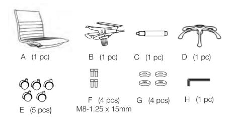
During assembly, hand tighten screws only. When the screws are in place, tighten completely.
