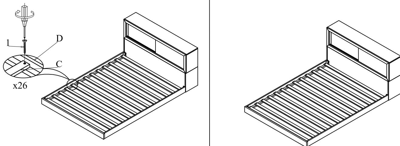
DO NOT TIGHTEN BOLTS UNTIL COMPLETELY ASSEMBLED /
