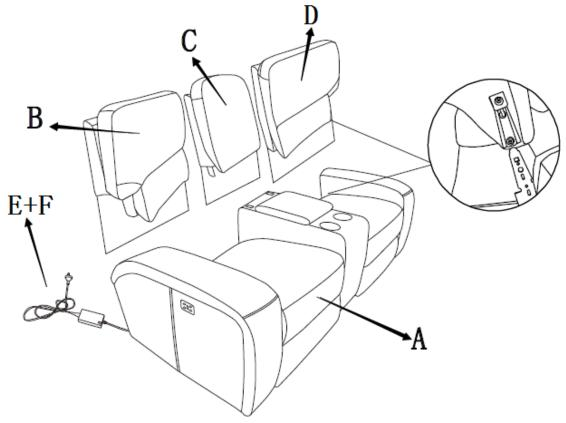
STEP#2 Attach the adapter and power cord to the position as shown in the drawing properly.
