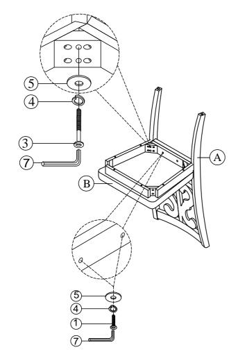
Step 2:Assemble Center bolts after corner bolts assembled.
