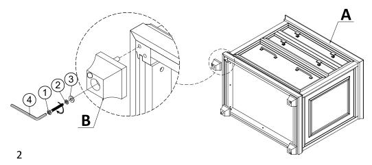
Turn the lateral file upright. Anti-tip hardware kit must always be used to prevent the case from tipping. Attach anti-tip restraint at top of the case inline to meet attachment on wall. Screw anti-tip into wall stud or use appropriate anchor for the type of wall if not drywall. Adjust leveler if needed.
