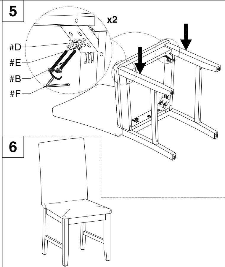
Tips: Turn chair upright on a level surface. Level the chair and tighten all bolts with the Allen Wrench.
