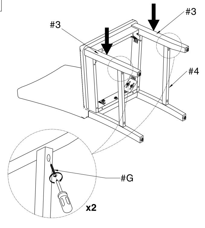
IMPORTANT: PRESS DOWN the front legs (#3) when securing with side stretchers (#4) using screws provided (#G) to avoid the gap between legs and stretchers.
