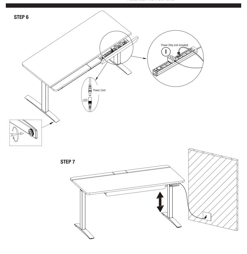
**STEP 6** Adjust levelers if needed to level desk. Connect Power Adapter (I). **STEP 7** Factory reset is required for first time initialization.
