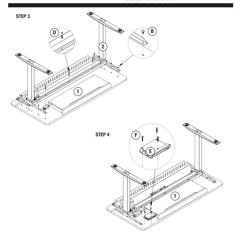
**STEP 3** Place Desk Top (1) upside down on a soft, non marring surface. Carefully place assembled Frame (2) onto Desk Top (1) and align mounting holes. Secure assembled Frame (2) to Desk Top (1) using eight Machine Screws (B) for Supports (3 & 4) and three Machine Screws (D) for center of Frame (2). **FULLY TIGHTEN ALL SCREWS USING ALLEN WRENCH (C).**
