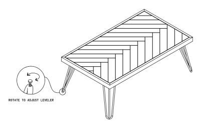
IF TABLE IS NOT LEVEL ON YOUR FLOOR, PLEASE ADJUST LEVELERS ON UNDERSIDE OF LEGS (B).
