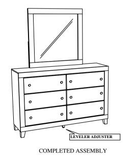
NOTE: MUST TIGHTEN SCREWS PERIODCALLY WITH USE SCREW WILL BECOME LOOSE CHECK TIGHTNESS OF ALL SCREW EVERY 6-8 WEEKS.
