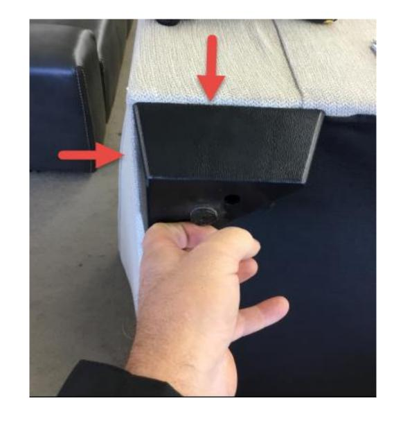
PUT THE SCREWS IN THE HOLES IN THE FEET. USE A PHILLIPS SCREWDRIVER, OR DRILL TO TURN THE **SCREWS INTO THE WOOD FRAMING** UNTIL THE SCREWS are TIGHT.
