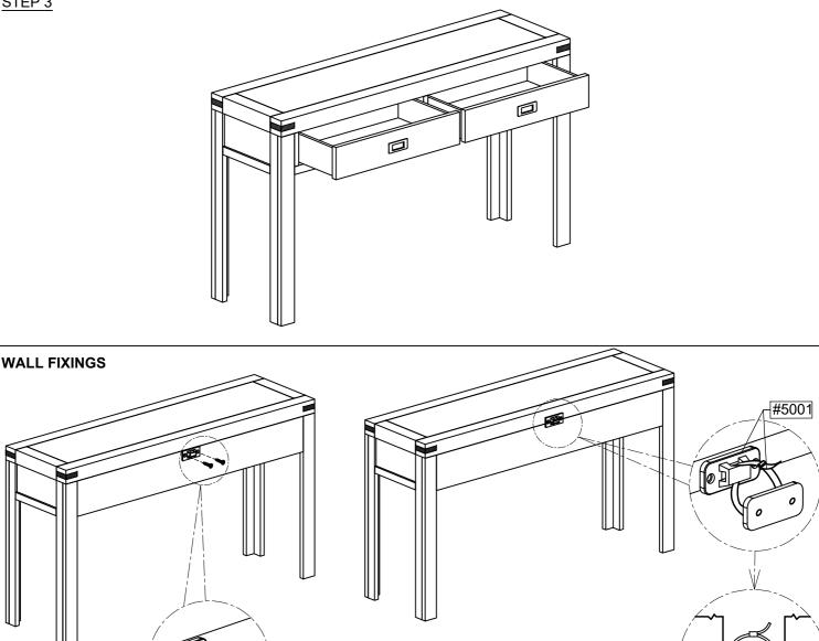
This wall fixing is provided for your safety and we recommend that once in position the unit is secured to the wall for extra stability
