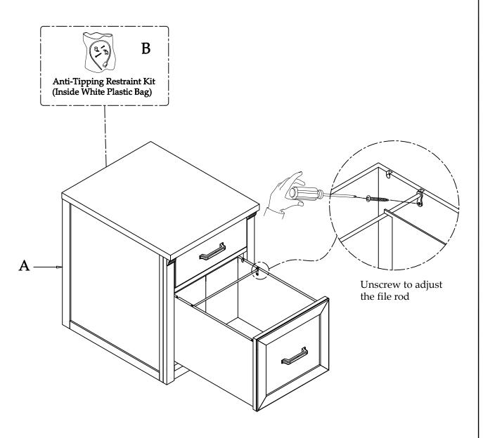
For product and personal safety, Anti-Tip Restraint Kit has been included with this cabinet which can help to minimize the risk of the cabinet accidentally tipping forward, if used and properly installed The File Drawer can be set up to use either Letter or Legal size hanging file folders using the File Rods installed in the file drawers.
