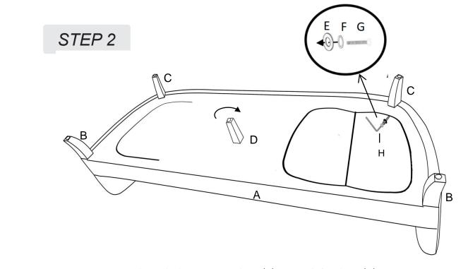
Insert 2 pieces of each Spring Washer (F), Metal Gasket (E) into 2 pieces of Bolt (G) as shown. Use Wrench (H) to tighten all the Bolts for the legs(B&C).
