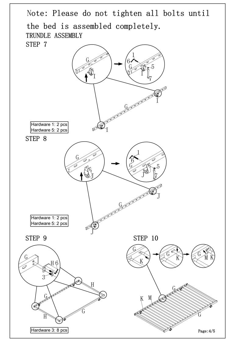
Note: Please do not tighten all bolts until the bed is assembled completely.
