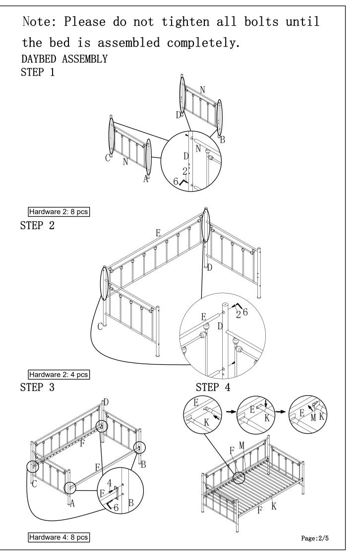
Note: Please do not tighten all bolts until the bed is assembled completely.
