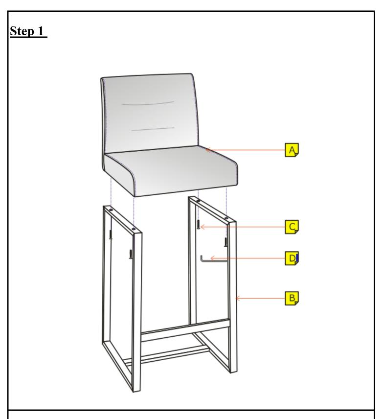
As the picture shows. Tighten the screws.
