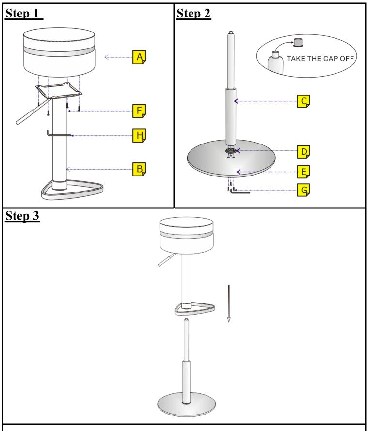
In order to activate the gas hydraulic, it is important that once you have assembled the stool that you raise the lever and bounce your weight up and down on the stool and then lift your weight off with the lever still raised and the stool should begin to rise.
