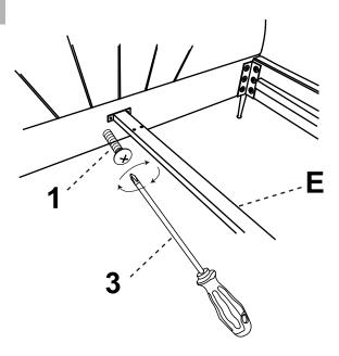
>Attach the center support bar as shown.
