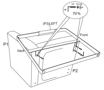
Step4.70% tighten bolts (H2) with allen wrench (H6) as illustration below.
