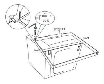
Step5.Turn the chair over, put on the leg, 70% tighten bolts (H2) and washers (H3 and H4) with allen wrench (H6) as illustration below.
