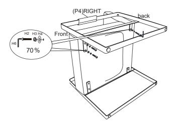
Step6.70% tighten bolts (H2) with allen wrench (H6) as illustration below.
