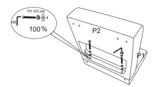
Step2. Tear off the cover on the gasket, paste the gasket on both ends of the foots as illustration below.
