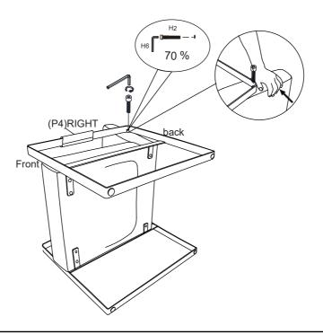
Step7. Fully tighten the bolts as illustration below.
