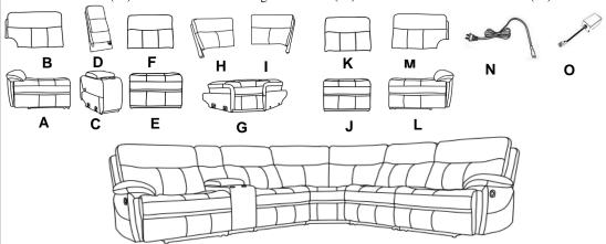
Step 1: Remove the transformer boxes(N&O) which are tied to the steel mechanism motor at the bottom of A,J and L.
