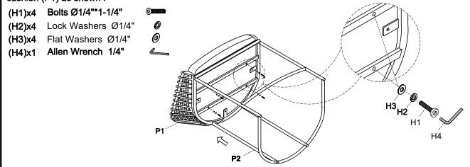
Step 2: Securely tighten all bolts with Allen wrench(H4), turn the assembled table to an upright position. Assembly is complete. Failure to follow these instructions may cause the bolts to misalign during assembly.
