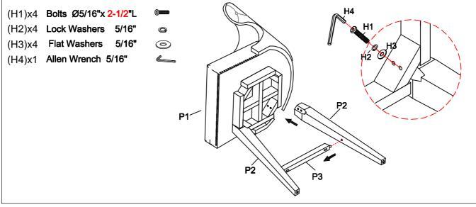
Step 2. Loosely Insert front stretcher (P4) between the two legs (P2), then attach the third leg (P2) to the bottom of chair top (P1) using bolt (H1), lock washer (H2) and flat washer (H3) as shown below.
