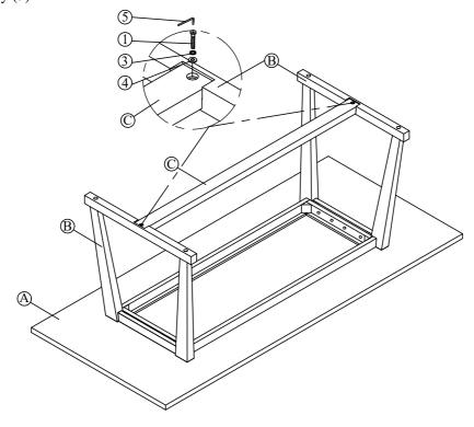
Step 3: Tighten all Allen Bolts so that the table does not wobble and turn up table on upright possition on level surface.
