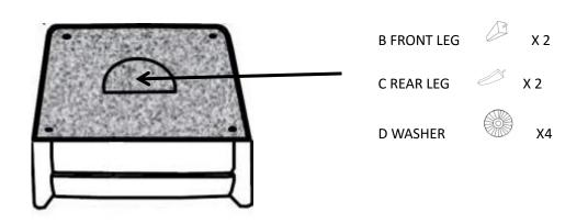
Step 2: Insert the washer onto the top of the legs, rotate the legs to tighten it. Rear leg curves must face outward.
