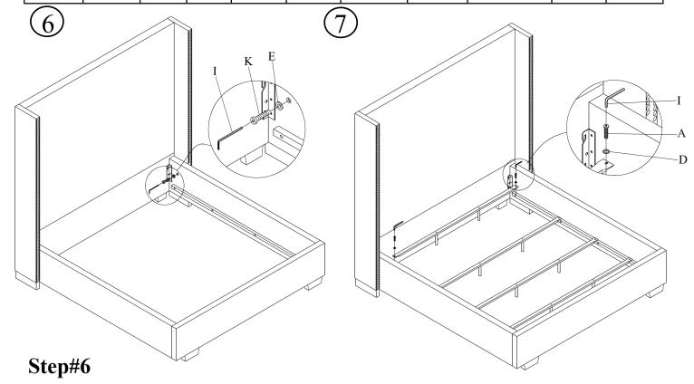
Attach wings through side rail finger tight, using Wrench(I), Bolt (K) and Washer (E) Tighten secure wings (6 bolts) with Allen wrench until snug.
