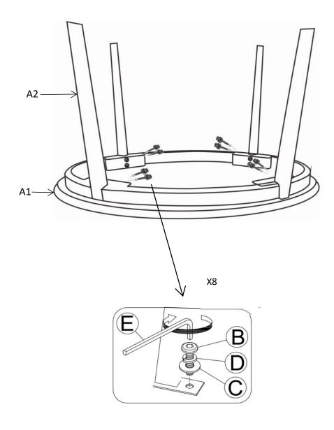
During assembly, hand tighten screws only. When all screws are in place, then tighten completely.
