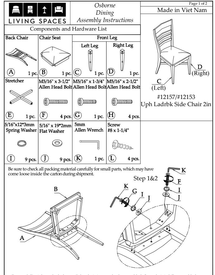
Do not fully tighten the bolts until the chair is completely assembled. Once chair is fully assembled, set the chair upright on a flat surface until it sits levels and then tighten all the bolts with the Allen Wrench provided. Attach all Velcro strips to the seat frame rails. Attach all Velcro strips around legs.
