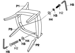
ADDITIONAL NOTE ABOUT SAFETY: BOLTS MAY LOOSEN DURING NORMAL EVERYDAY USE. THEY SHOULD BE PERIODICALLY INSPECTED AND RE-TIGHTENED TO PREVENT DAMAGE OR INJURY. ALWAYS CHECK TO ENSURE THAT ALL HARDWARE IS KEPT TIGHTENED.
