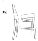
Step 5: Lock the seat (P5) to the back frame (P4) using Allen Wrench (H4) to loosely tighten bolt (H1), lock washer (H2), flat washers (H3) as below illustration. Loosely tighten the screw (H5) with the screw driver (H6) to lock P1 and P2 to the back legs (P4) as illustration below.
