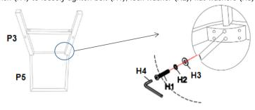
Step 3: Insert P1 and P2 to the front leg frame(P3),lock the footrest to the front legs, loosely tighten the screw (H5) with the screw driver (H6) as illustration below.
