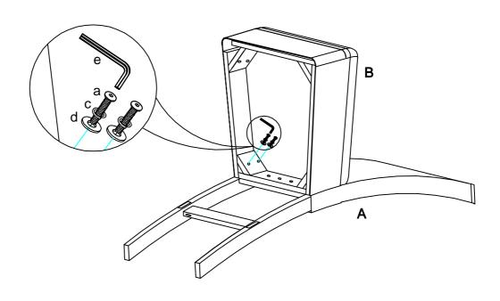
Step 3. Insert the right stretcher (D) to the leg of chair back (A) according to the label "R" at the hole in the leg and the front end of right stretcher (D). Loosely attach the front leg (F) to the bottom of seat cushion (B) and the stretcher (D) using bolt (b), lock washer (c), flat washer (d) and Allen wrench (e). Do not tighten the screws at this time.
