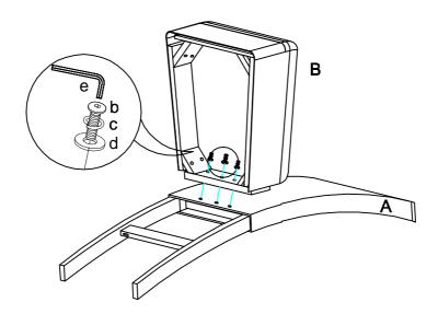
Step 2. Attach the seat cushion (B) to the leg of chair back (A) using bolts (a), lock washers (c) and flat washers (d). Loosely tighten with Allen wrench (e).
