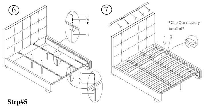
Locate bed in final position before attaching center supports.
