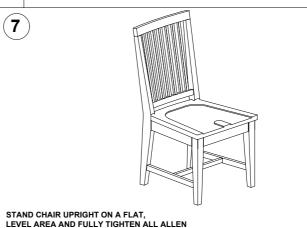
STAND CHAIR UPRIGHT ON A FLAT, LEVEL AREA AND FULLY TIGHTEN ALL ALLEN BOLTS WITH THE ALLEN KEY
