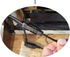
Check connection security and integrity of motor's 2-pin cable
