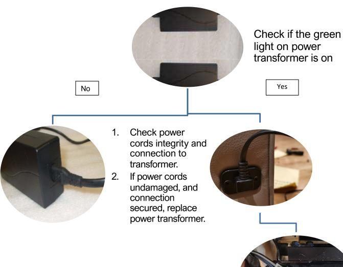
Check connection security and components integrity on DC socket and power cable.
